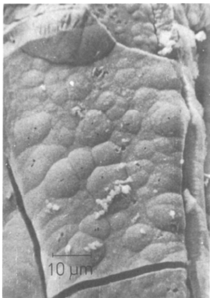
Fig. 2. SEM micrograph of polypropylene–nickel auxiliary electrode (No. 5) prepared by electrochemical method.
