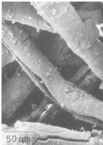
Fig. 2. SEM micrograph of polypropylene–nickel auxiliary electrode (No. 5) prepared by electrochemical method.
